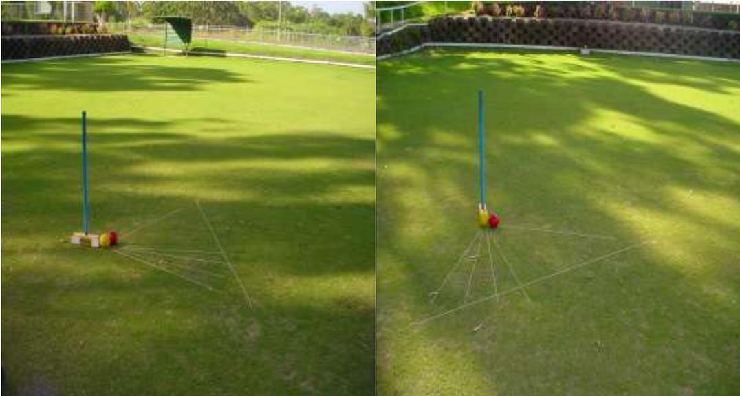
**Photos above show the string lines, angles, mallet with carbon papers attached and ball set up used for the tests.**
